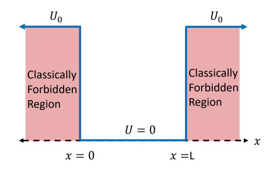
Since the potential is not infinite, the wavefunction extends into the walls
